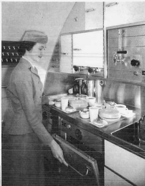
*Unique* features include colorfully modern galleys; plastic window shades, both smoke-tinted and opaque; passenger service unit above each row of seats, containing air inlets, individual reading lights, etc. The 707 interior has been under development since 1952.
